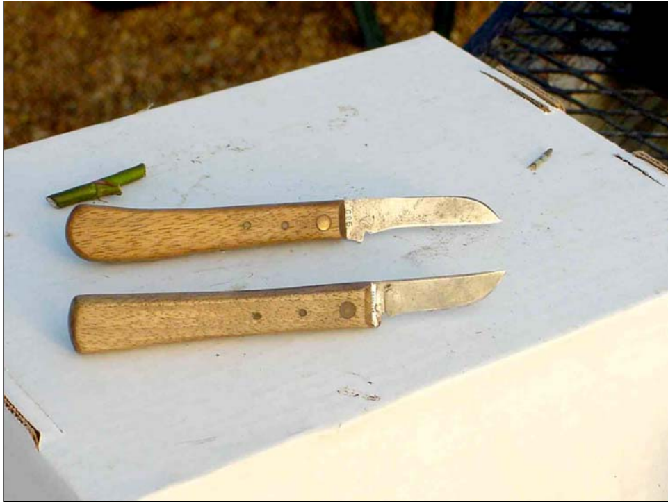
Grafting knife with a straight blade and budding knife with a curved blade. The blades are thin and make a clean, smooth cut.
