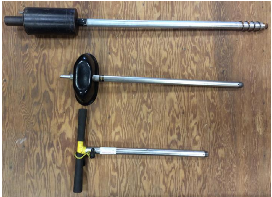
Figure 1. Selecting a good hay probe is a very important component of collecting a representative sample in the bale and in the hay lot. Probes can be either hand-powered or power-driven. Figures are for reference purposes only and reference to commercial products or trade names is made with the understanding that no discrimination or endorsement is intended and no endorsement by Mississippi State University, Mississippi Agricultural & Forestry Experiment Station or Mississippi State University Extension Service is implied.
