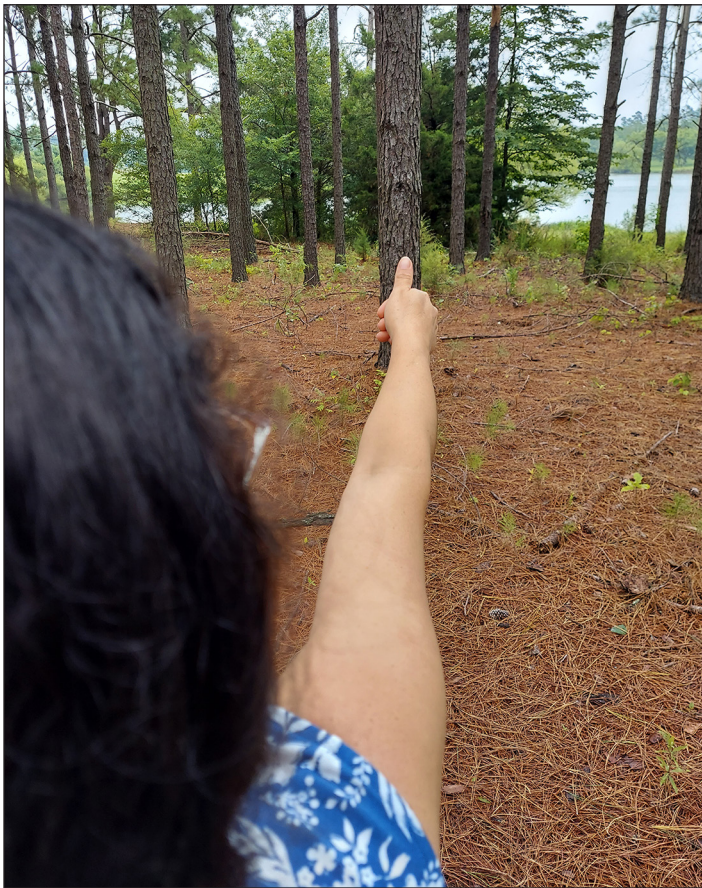
Figure 3. A thumb can be used to project an “imaginary” horizontal angle, which can be equated to a basal area factor (BAF). If you extend your thumb some distance from your eye, assuming the vertex of the angle (where the angle begins) is located in your eye, then an imaginary horizontal angle is projected out to your thumb and beyond (depicted on the right). This is the same approach used for stick angle-gauges, Cruz-All tools, etc. Depending on the width of your thumb and your arm distance, you can use this approach to generate your own BAF. Whenever the width of the thumb is smaller than the tree image at 4.5 feet above the ground (diameter at breast height) the tree is “in.” To obtain basal area per acre, just multiply the number of “in” trees at each point by your thumb-specific BAF.
