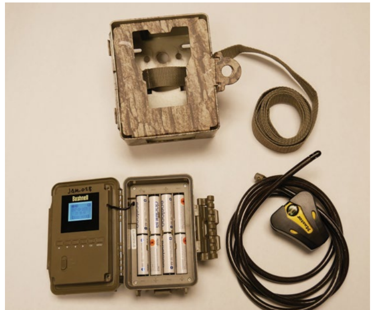
Figure 17. Camera trap components, including a camera with eight disposable batteries, security box and strap, and cable lock. (Photo by Eden Blackwell/University of Alabama)
