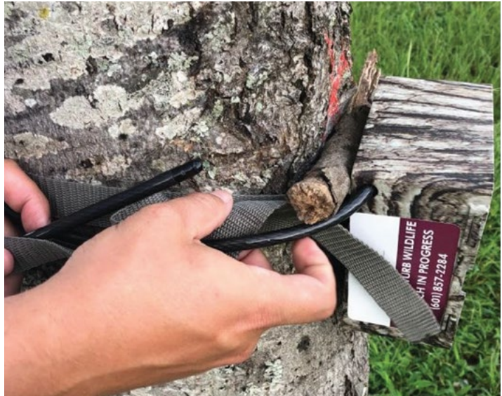
Figure 8. Cable cords and camera straps are interwoven to avoid triggering the camera. The camera is angled downward to capture small mammals low to the ground and avoid human faces. (Photo by Matthew Oswald/South Carolina Department of Environmental Services)
