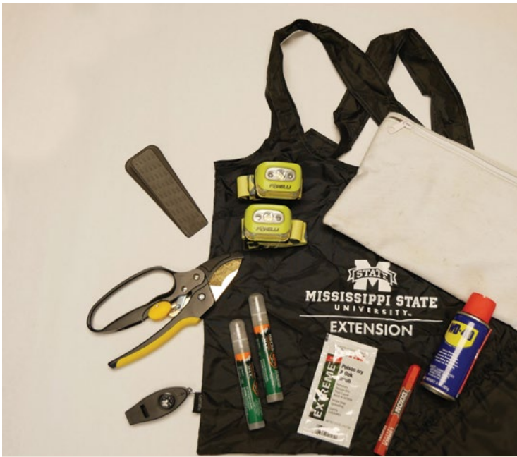
Figure 18. Field bag and contents of miscellaneous tool kit, including shears, insect repellent, and a lumber crayon. (Photo by Eden Blackwell/University of Alabama)
